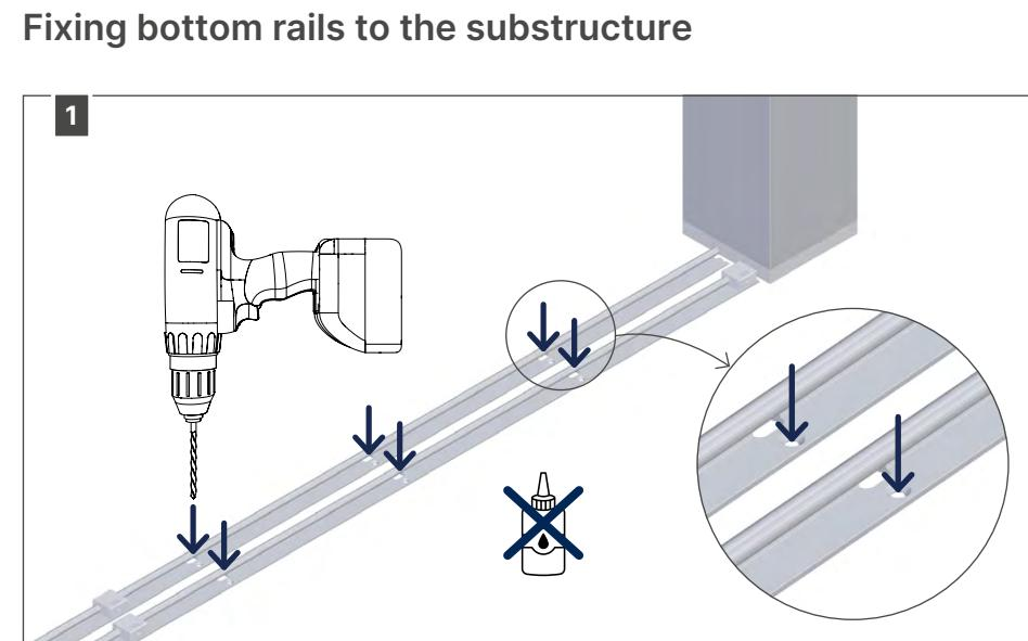
Use screws that are suitable for the surface, e.g. DIN 7982 CH - ST4.2×13 (not supplied).
