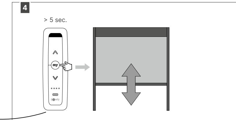
If the result of your check in step 3 is not correct, press for more than 5 seconds on the MY button on the remote until the Fix screen makes a short up- and downward movement. Check that step 3 is now giving correct results.
