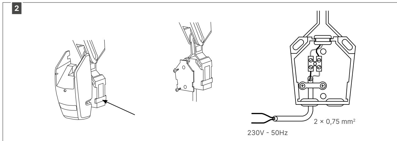
Open the wind sensor and connect a 230 V power supply.
