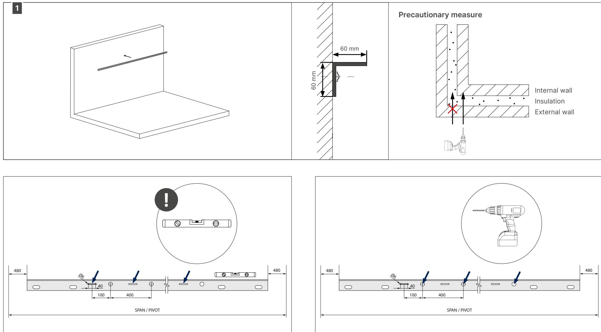
Provisionally secure the L-profile via the slotted holes.
