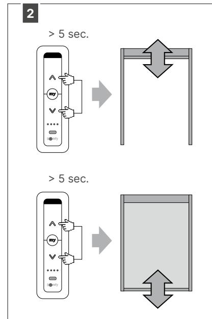
Press more than 5 sec. on the UP- and DOWN-button till the Fixscreen makes a short movement.
