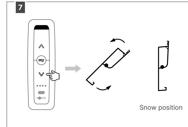
Close the blades until they return to a completely vertical position (this is the preferred snow position). To do so, hold down the DOWN button.
