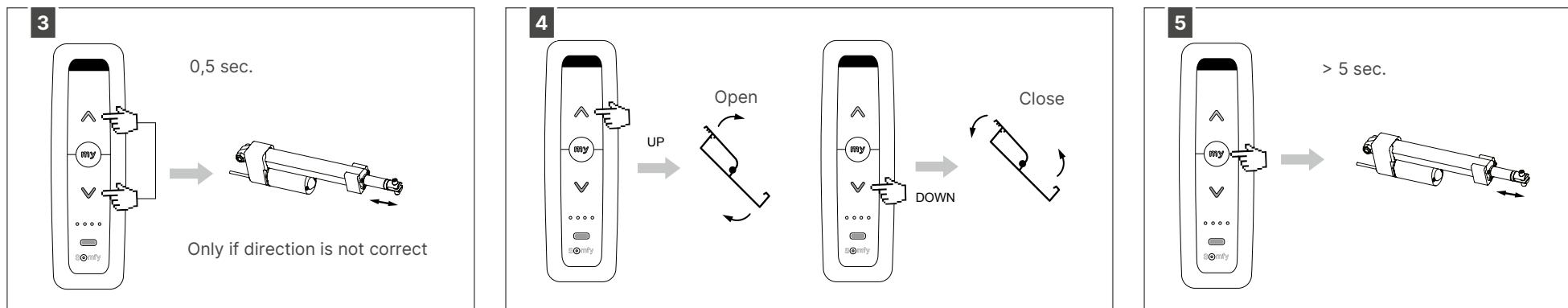
Press the UP and DOWN buttons on the remote simultaneously (briefly). The motor drive makes a short outwards and inwards movement for confirmation
