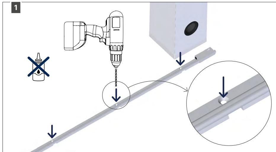
Use screws that are suitable for the surface, e.g. DIN 7982 CH - ST4.2×13 (not supplied).
