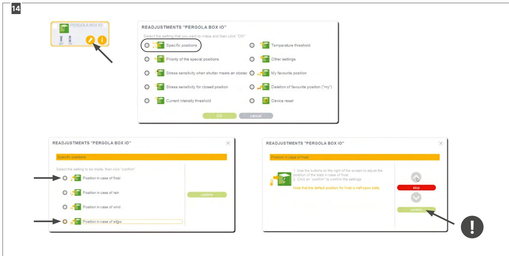
Under the 'specific positions' section, you can set the required position in case of frost and snow.
