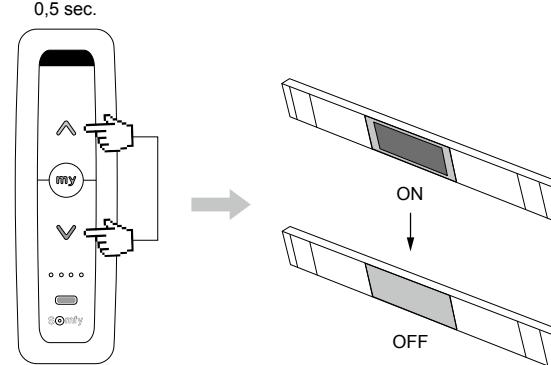
Press the UP and DOWN buttons briefly at the same time on the hand-held remote until the heating element briefly switches on and then switches off.
