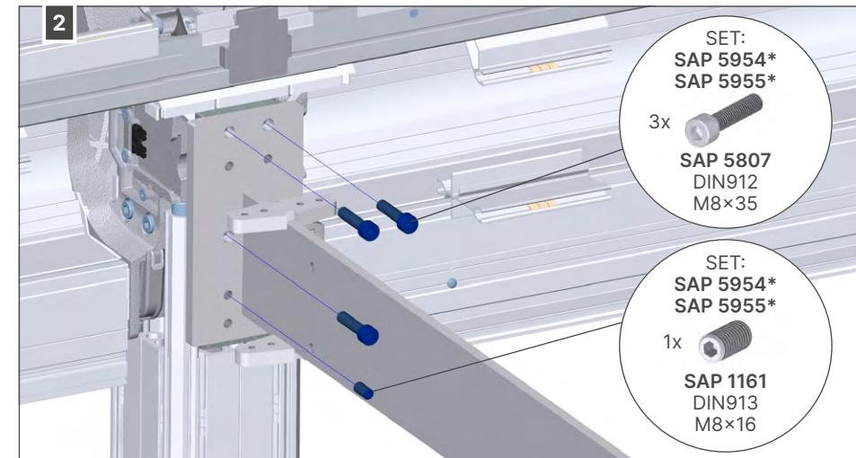
\* SAP 5954: joining knife bracket pivot - SAP 5955: joining knife bracket span
