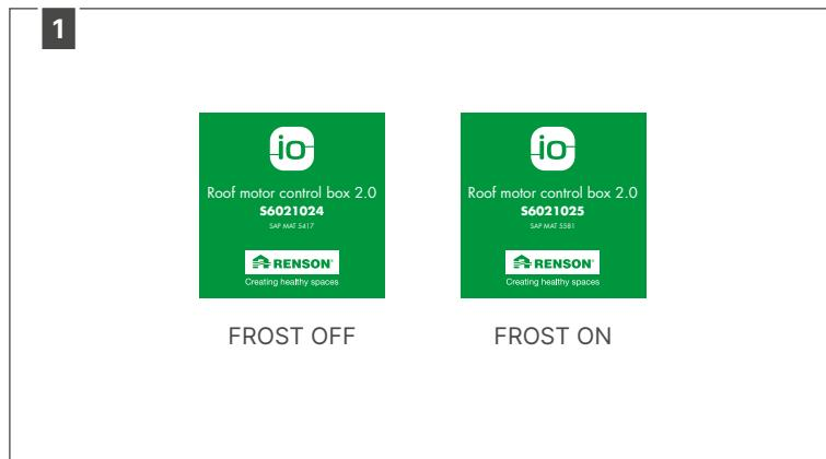
When ordering the product, you were given the option of selecting the motor control with active or inactive frost/snow protection. The item number on the label of the motor control will tell you the factory setting of the motor control;
