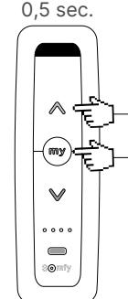
Press (shortly) the MY and the UP buttons on the remote simultaneously (shortly) to confirm this bottom end point. The Fixscreen goes automatically back up.
