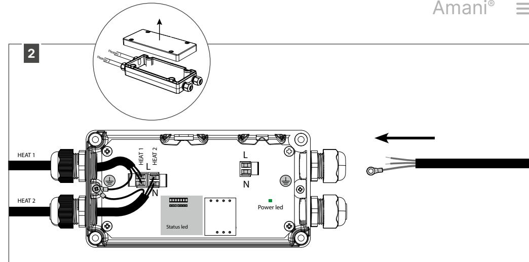
To do so, first remove the transparent cover of the receiver and insert the power cable through the open cable gland into the receiver.
