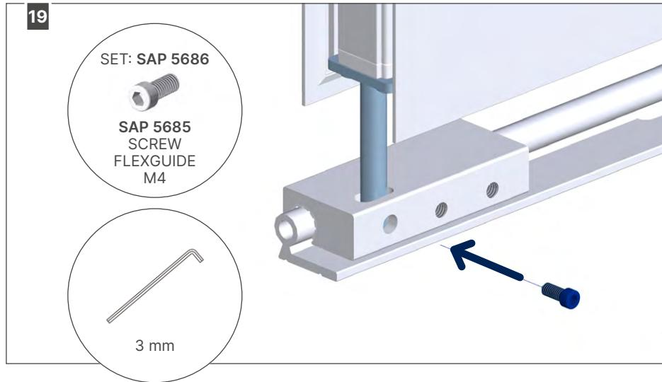
Installing position lock to place folding panels in stacking position
