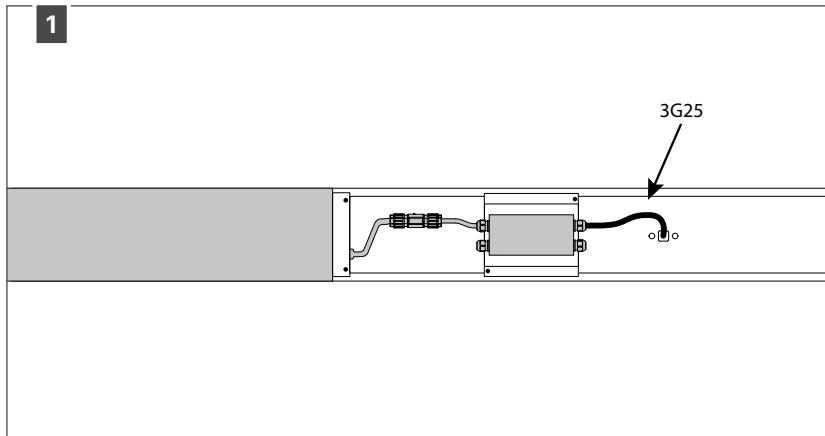
If a receiver is provided, plug the power cable into the receiver.
