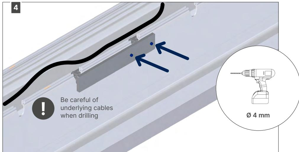
Note: push the jig down while drilling.
