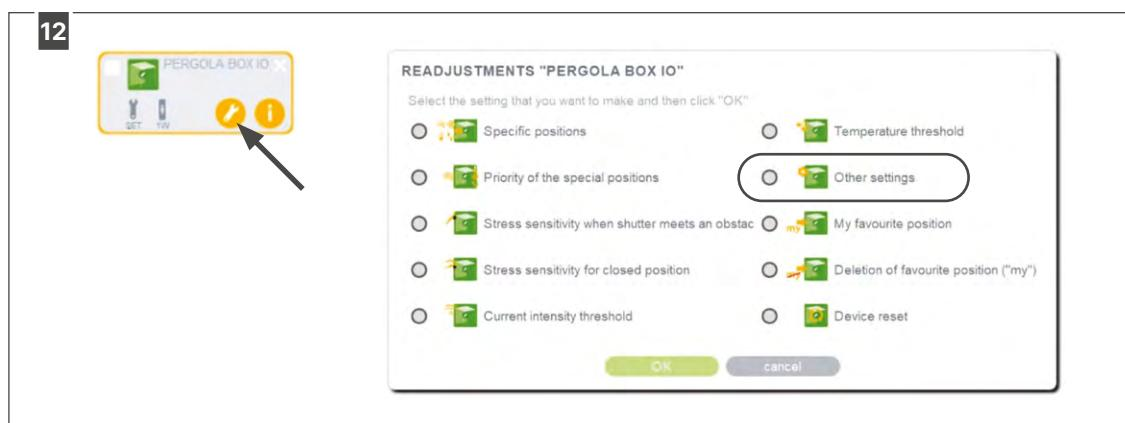
Using the settings button (spanner icon), you can view the settings of the Pergola Box IO. Under the 'Other settings' section, you can turn the frost/snow protection on and off.
