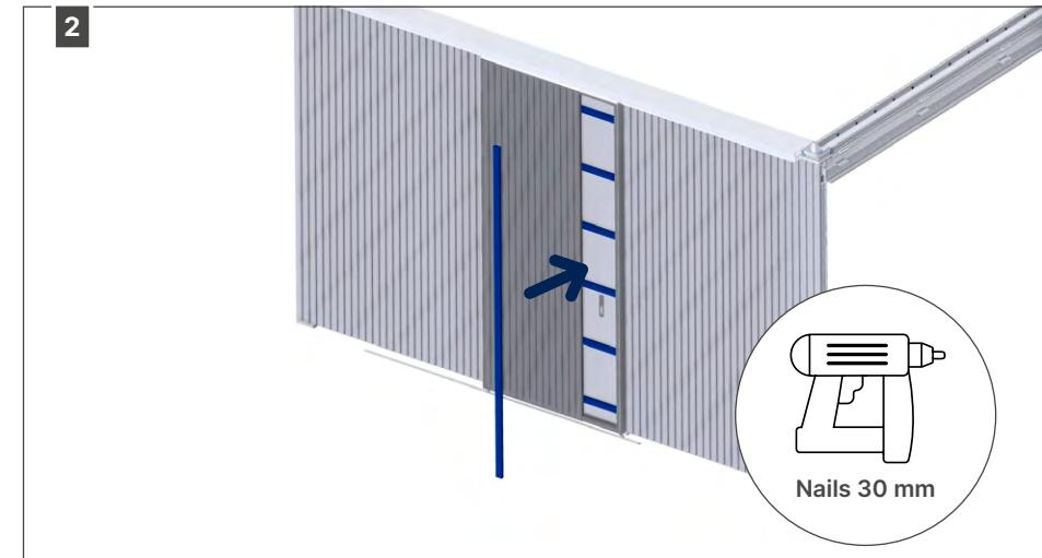
\* In case the fixed wall with door is positioned under the couple beam, the length of the wood is equal to the passage height – 40 mm (length wood = PH – 40 mm).
