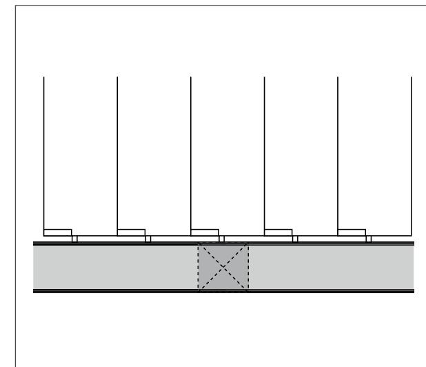
A beam is partially interrupted by an intermediate or shifted column.
