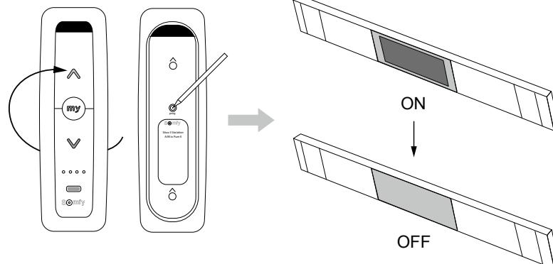
Press the PROG button briefly on the back of the hand-held remote. The heating element briefly switches on and then off to indicate that the hand-held remote is programmed in the Heating Receiver.
