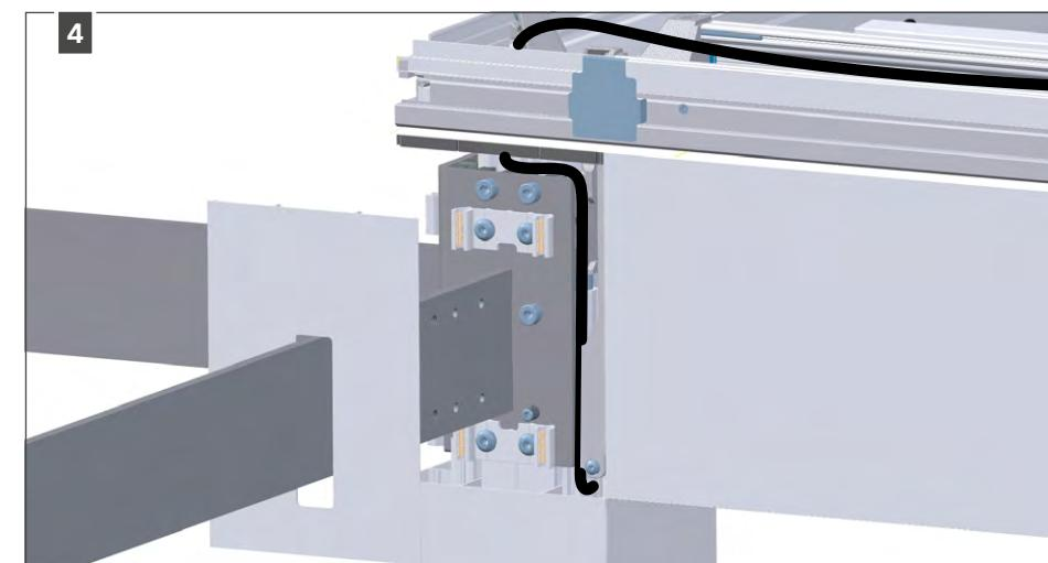
Slide the cable under the water funnel.
