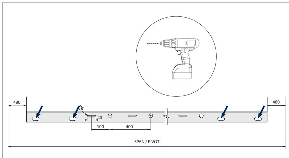
The consoles are mounted through the slots of the L-profile.
