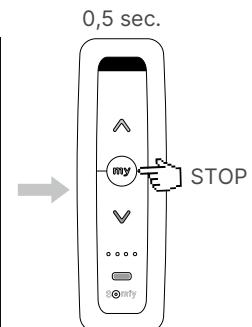
The Fixscreen goes automatically down. Press (shortly) on the MY button of the remote as soon as you have reached the desired bottom lower end point.
