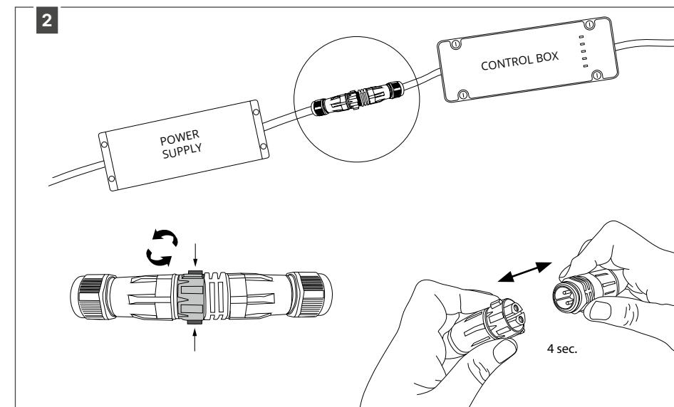
Disconnect the connector between the transformer and receiver for 4 seconds. Turn the screw with the 2 protruding wings.
