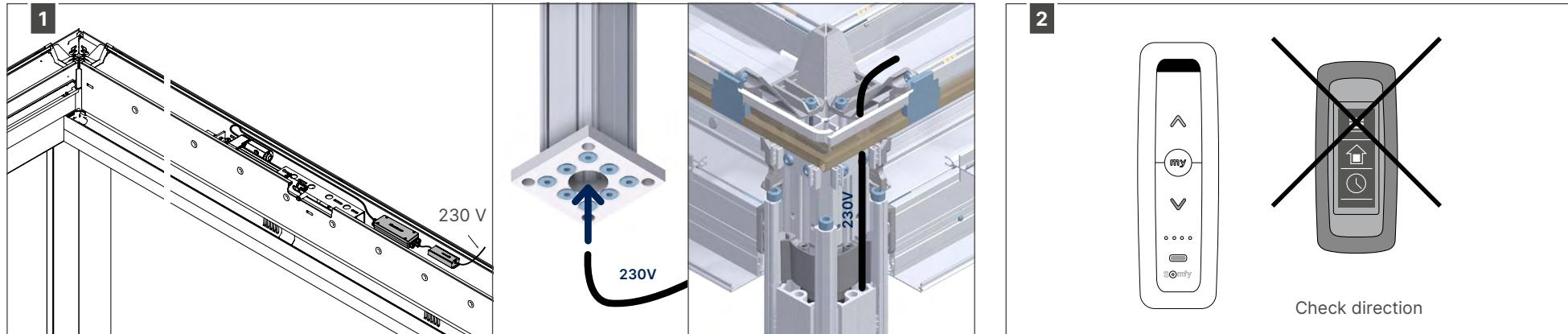
The motor control and power supply are already connected to the motor. First and foremost, connect the transformer to the main power (230 Volts AC).
