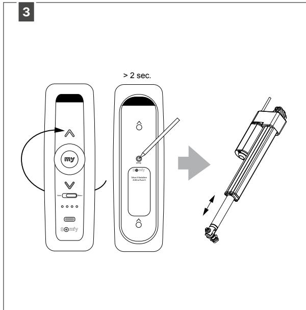
The wind sensor must be programmed. The motor must be in programming mode in order to program the Eolis wind sensor.
