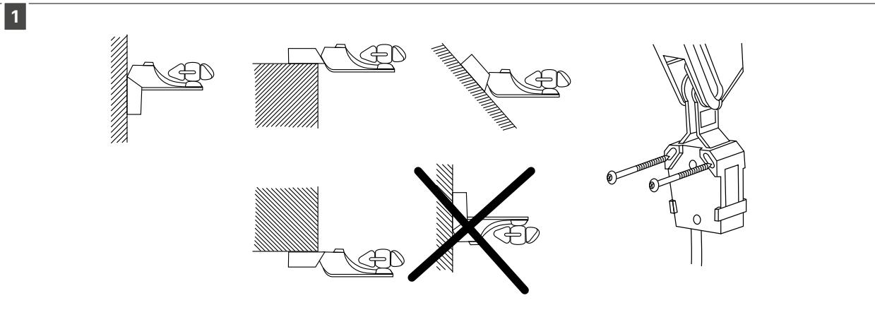
Position the Somfy Eolis wind sensor in an open place.
