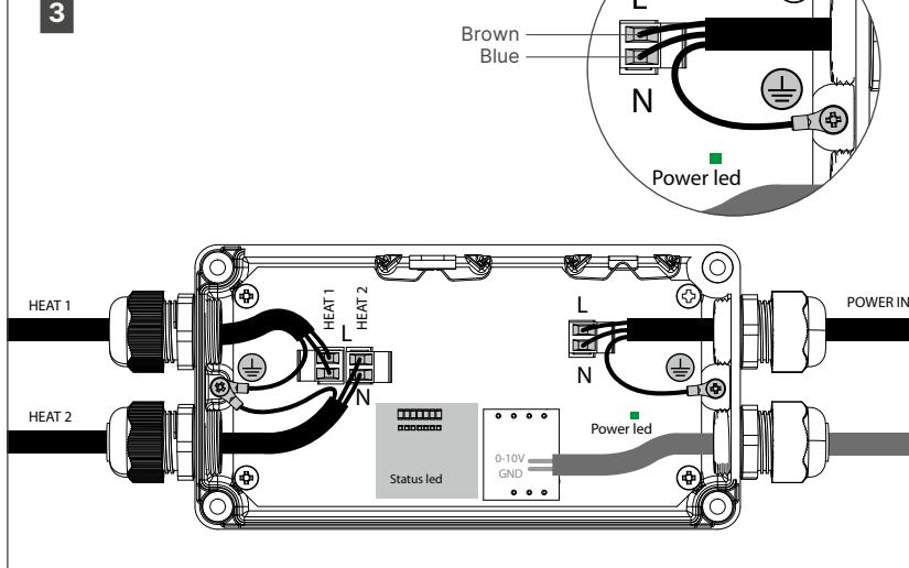
Connect the brown wire to the L terminal and the blue wire to the N terminal. Attach the cable eye (earthing) via the screw between the 2 right glands. Also connect the 0-10V control signal.
