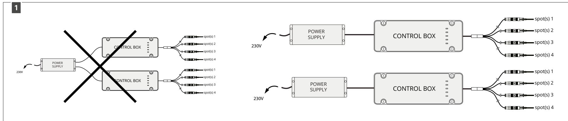
**Note:** If there are multiple controls, these must never be powered together.
