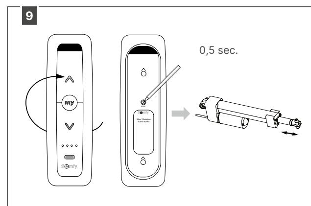
Press briefly on the PROG button on the rear of the Situo io remote, until the drive makes a short outwards and inwards movement. That confirms all settings.
