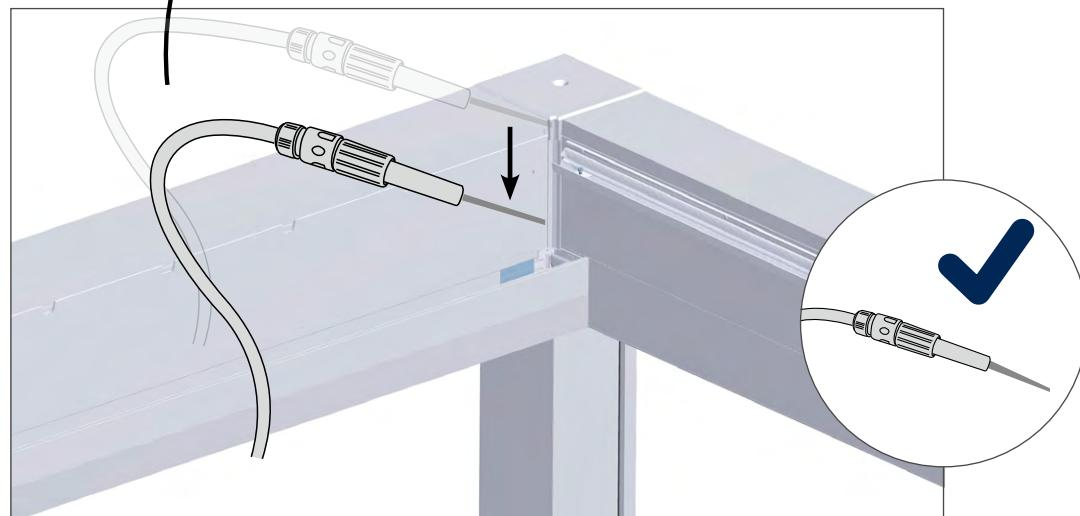
Test the nodes to ensure that they are watertight.
