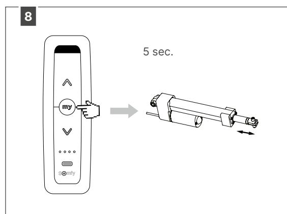
Confirm this vertical position (also referred to as snow position) by continuously pressing the MY button for 5 seconds. The motor drive makes a short outwards and inwards movement for confirmation.
