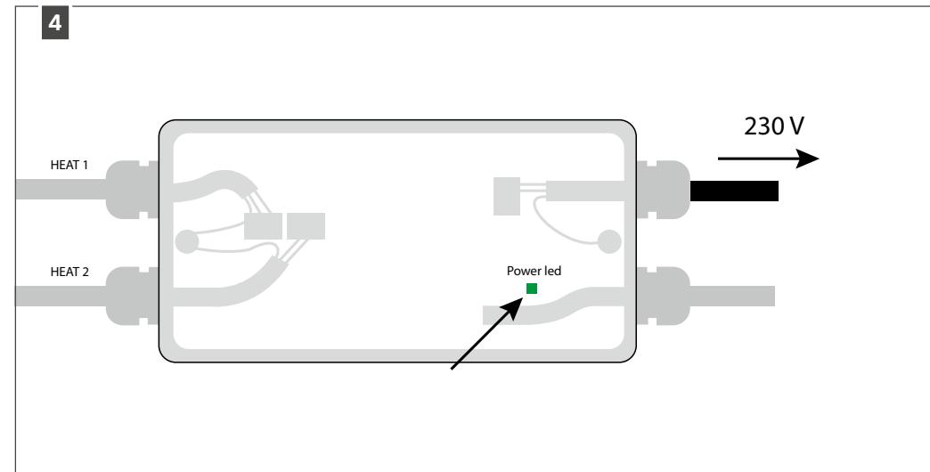
Then connect the power cable to the mains voltage (230 volts AC). The power LED in the receiver should light up green. This tells you that the receiver is effectively receiving voltage.
