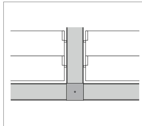
3 beams come together. A T-junction is a mechanical connection of 3 frame profiles - two span profiles and one pivot coupling beam or vice versa. This occurs with linked building types.
