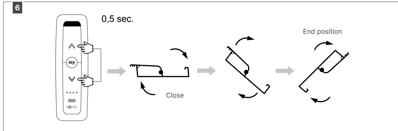
(Briefly) press the UP and DOWN button on the remote simultaneously. The blades will close completely and then automatically open completely (these are the end points).
