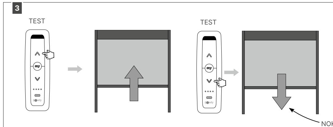
Check if, when pressing the UP button on the remote, the Fixscreen makes an upward movement. And check that, when pressing the DOWN button on the remote, the Fixscreen makes a downward movement. If so, you can proceed to step 5.
