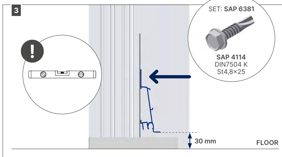
The support profile must be level. If the slope is slanted, the support profile must hang at least 30 mm from the floor.
