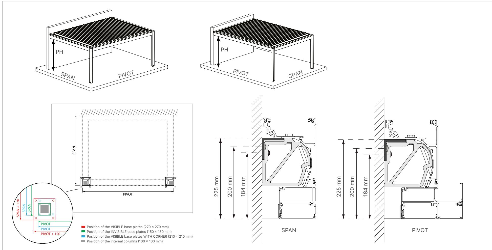
Determine the position of the L-profile and mark it on both sides of the wall.
