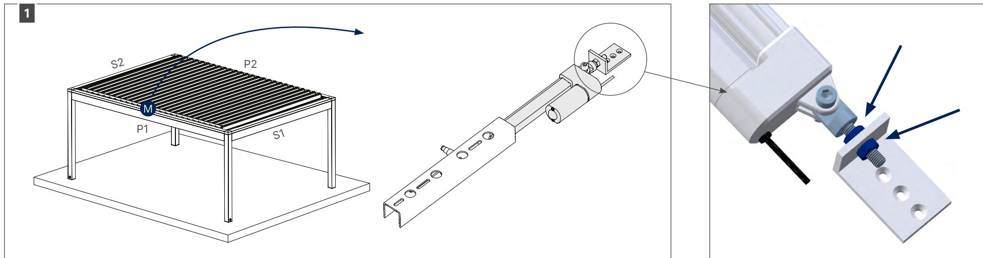
The position of the blade drive is adjustable if the blades are under too much tension or are not closed completely after closing,
