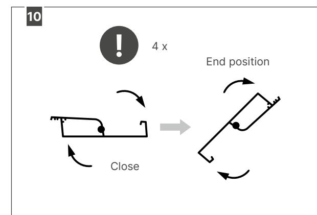
**Attention:** After setting the control for the louvred roof, it's important to fully open and close the roof 4 times.
