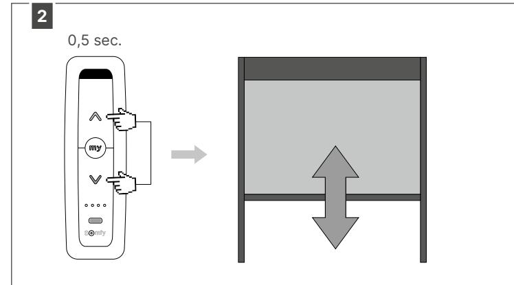
Press the remote's UP and DOWN button simultaneously (briefly).
