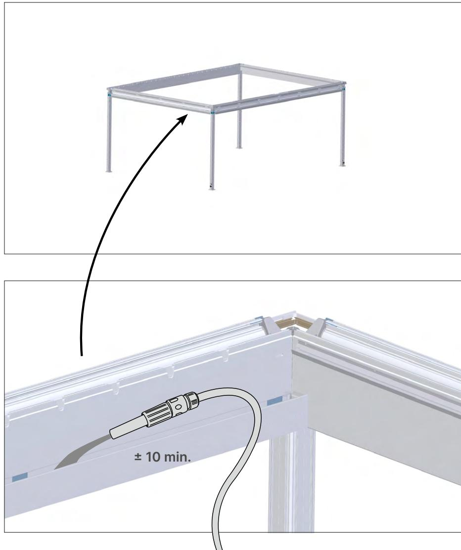
We recommend testing every installation for water infiltration prior to delivering. This can be done in a number of steps.
