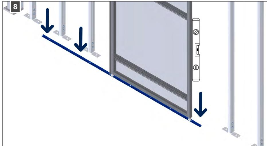
Secure the bottom rail. Use screws that are suitable for the surface, e.g. DIN 7982 CH - ST4.2×13 (not supplied).
