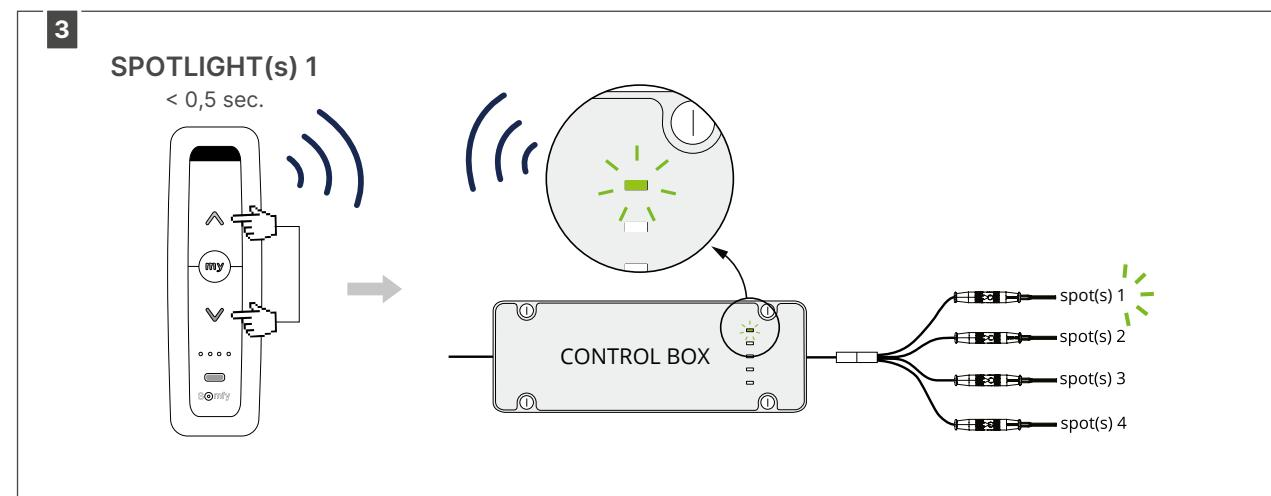
(Briefly) press the UP and DOWN button on the Situo IO remote control simultaneously. The spotlight connected to the first output will light up.
