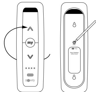
Press the PROG button briefly on the back of the Situo IO remote control. This confirms the setting.
