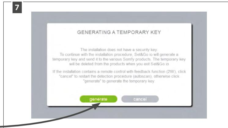
Skip this step if no two-way remote is connected.
