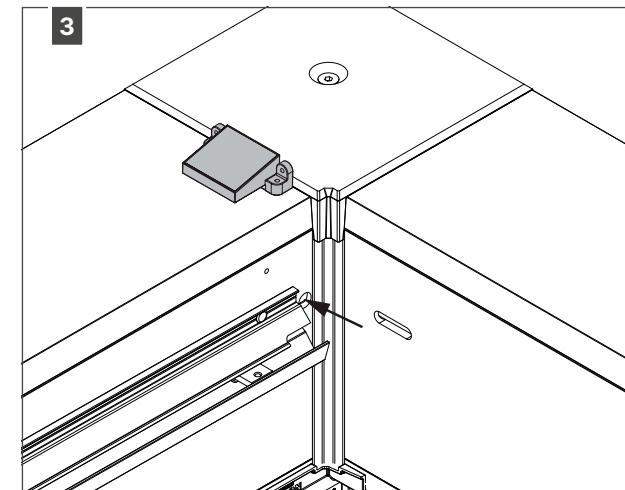
Feed the cable through the opening in the fixed blade.
