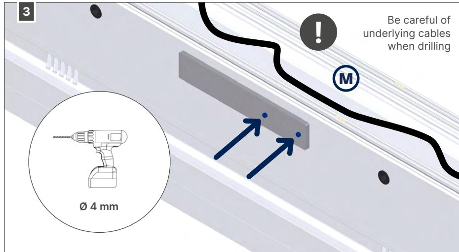
Note: push the jig down while drilling.
