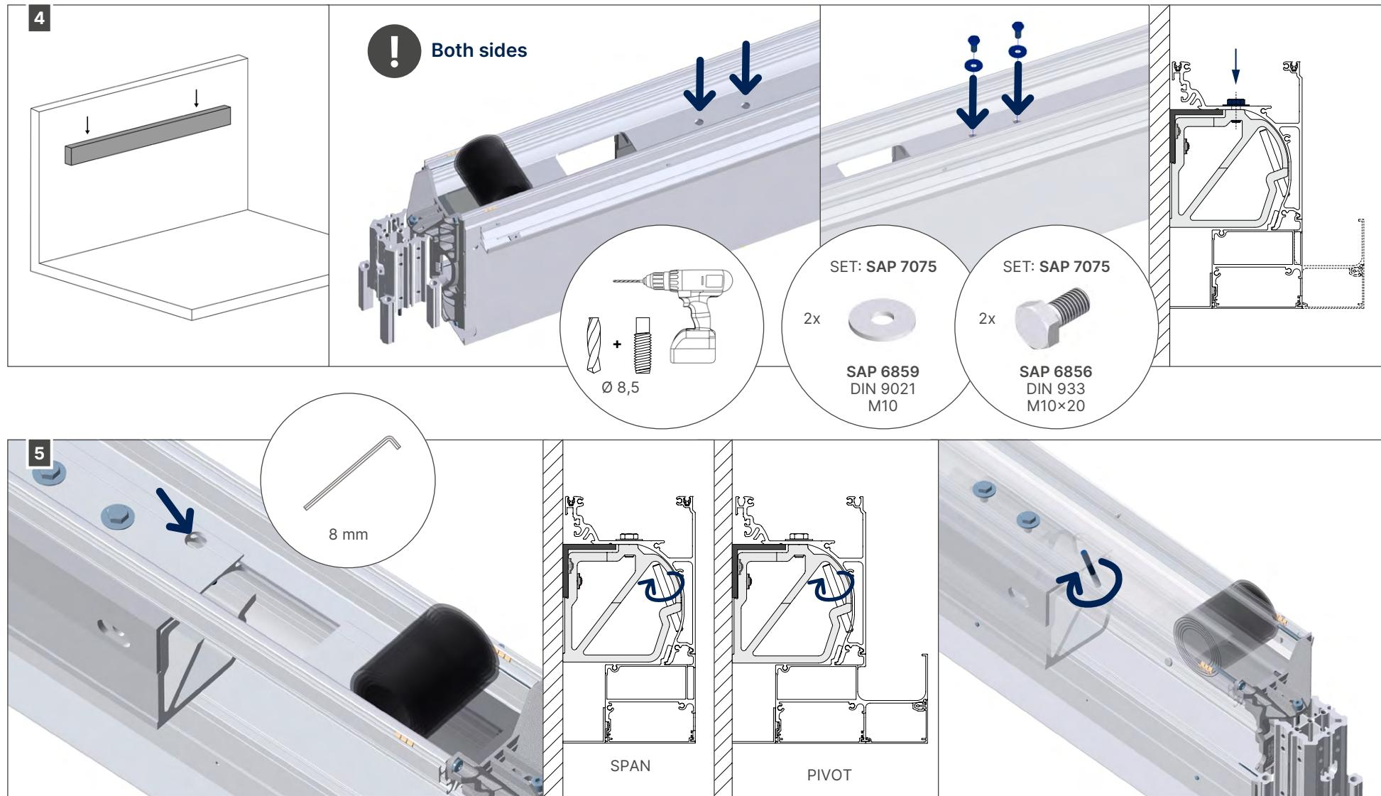
Tighten the adjusting screws in the consoles so they engage behind the hook profile. This provides extra security for the beams.
