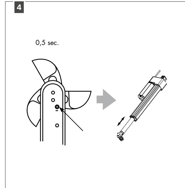
Press briefly on the 'program' button of the Eolis wind sensor. The drive makes a short outward and inward movement for confirmation. The wind sensor is programmed.
