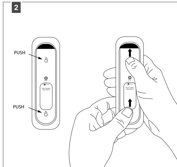
Remove the cover at the back of the remote control.
