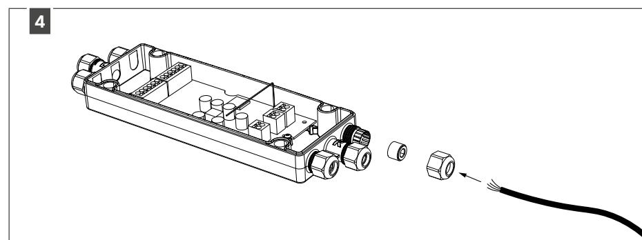
Open the cover of the connection box. Pierce the right grommet with the blue rubber. Put the cable of the rain sensor through this cable gland.
