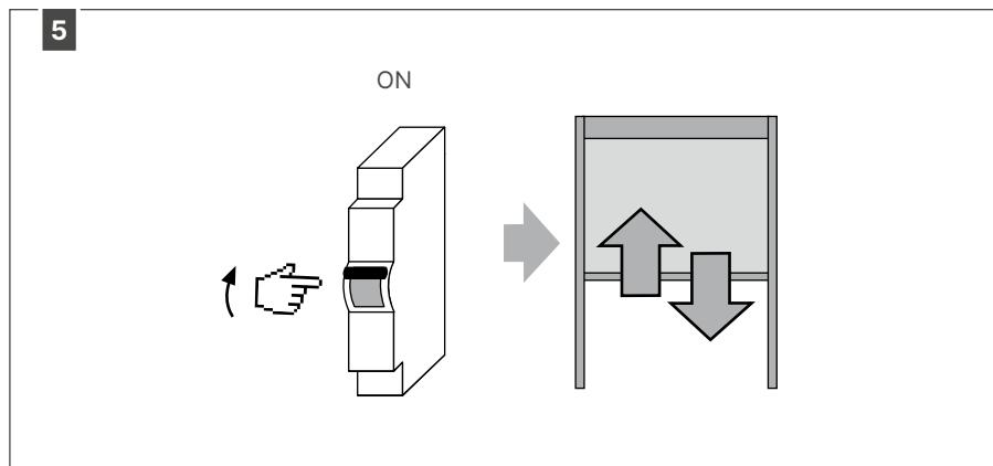
Switch on the power 230V. If the Fixscreen is in a position between the end points, it moves in the opposite direction from the last movement for about 3 seconds. If the Fixscreen is at an end point it makes a short up- and downward movement.
