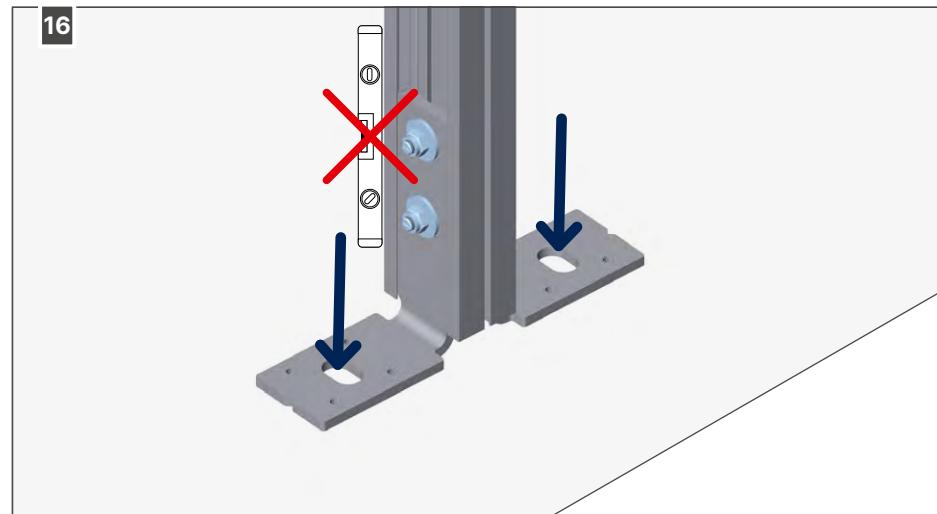
Secure the support posts. Use fasteners adapted to the relevant surface (to be provided by the installer).
