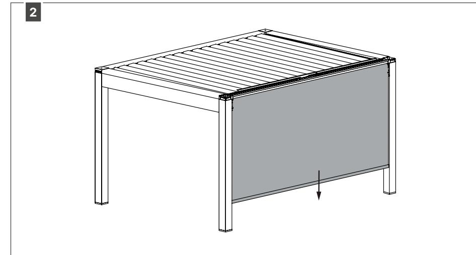
For ergonomic reasons, install the Fixscreen without the bottom bar. However, for specific configurations, mount the bottom bar first and skip steps 1 and 2. Then install the Fixscreen in the patio cover.
