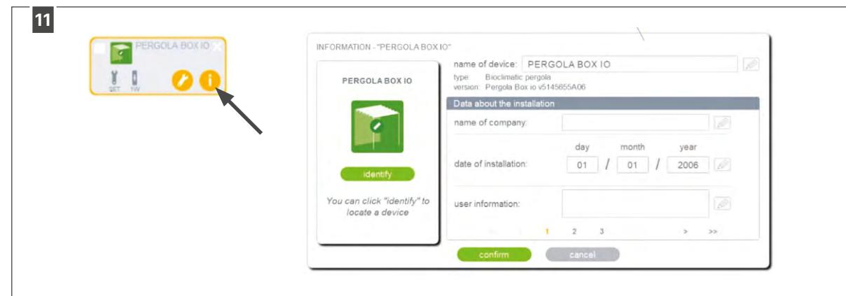
You can see the specifications for each device via the information button ("i icon"). These details consist of three pages (indicated at the bottom by 1/2/3). You can use this menu to assign a name to the device, view the connected remotes etc
