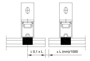
Locate the support structures as close as possible to the outer end of the blade. The clearance between the blade support and the end of the blade should not exceed 10% of the allowed free length of the blade.
