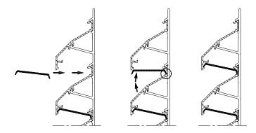
• Stainless wire mesh V2A in 2.3 x 2.3 mm, 6 x 6 mm, 10 x 10 mm or 20 x 20 mm mesh (supplied on roll) The mesh is fixed to the substructure or the support structures.
