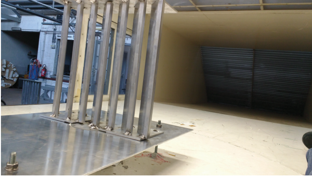
Figure 3: Example of the most set-up with array but without end plate, which was the most commonly tested configuration. The photograph is taken looking downstream towards the exit louvres.
