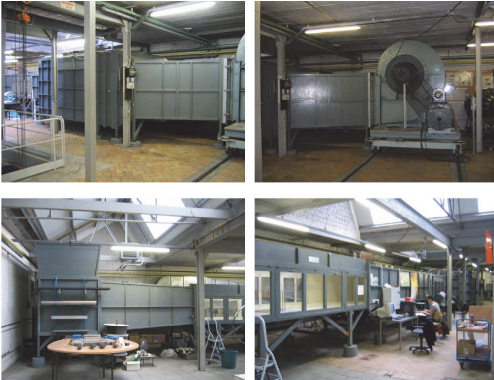
Figure 1: General overview of the wind tunnel. Clockwise from top left: the settling chamber, the centrifugal blower, the test section, and the diffuser with exhaust.
