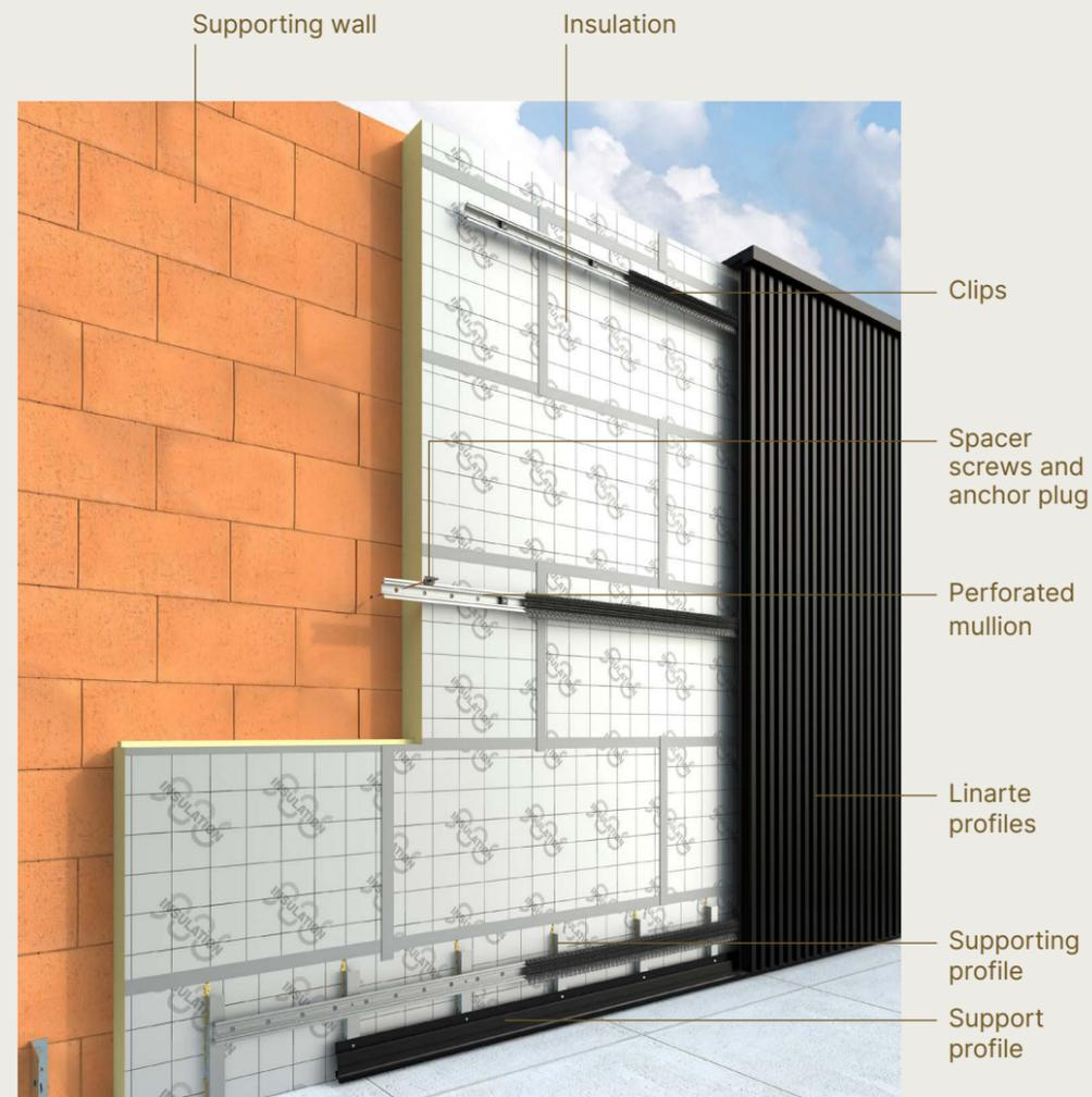
With the patented fixation system, the mullions can be directly affixed to the substructure. Compared to the traditional system using a wooden support structure, this method is more advantageous because of the lower material cost and quicker installation time. Thanks to the direct fixation, there are fewer thermal bridges, the total system depth is smaller, and you have a more sustainable solution.
